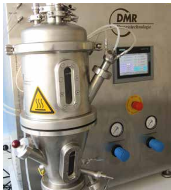
Figure 1. Laboratory-scale fluidized bed dryer, granulator and coater.
