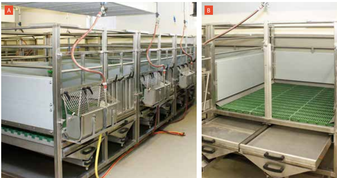
Figure 1. Metabolic pens used at the Center for Applied Animal Nutrition in Tulln. A) Front and side view with feeders and drinkers in the front door B) Inside view with slatted floor, collection area with screens and trays.
